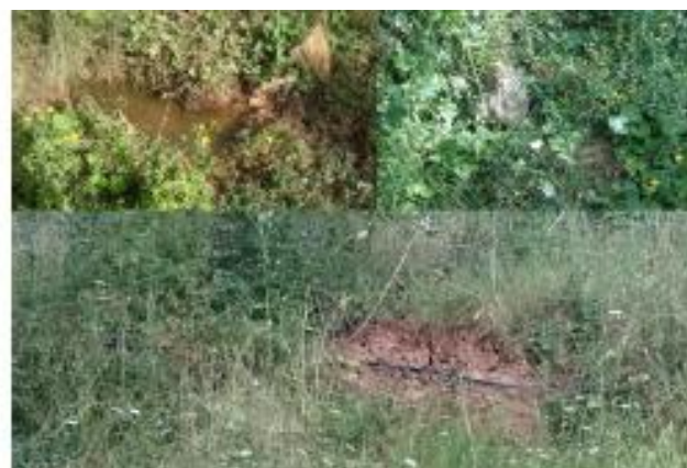
Figure: Typical shallow failure due to suffusion of soil particles (left) and damaged water supply system with uncontrolled irrigation of landslide area (right)
